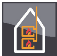
Decentralized multiple fireplaces connected to same chimney
